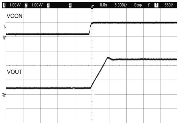
Figure 25. V_{OUT} Rising Transition 0.5 V to 2.5 V, V_{IN} = 3.7\text{ V}
