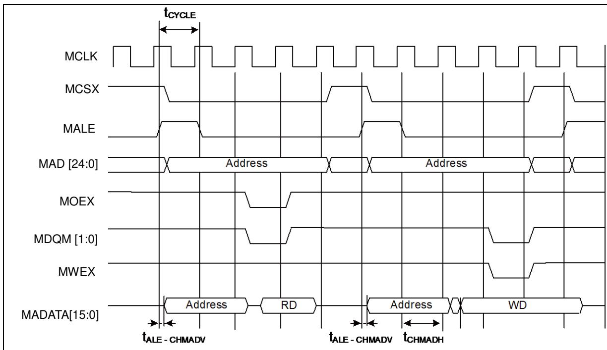
**Multiplexed Bus Access Synchronous SRAM Mode**
