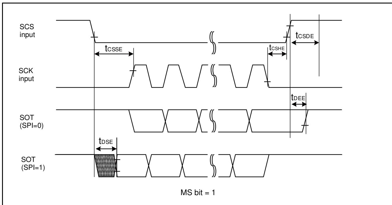
**When Using High-Speed Synchronous Serial Chip Select (SCINV = 0, CSLVL=0)**
