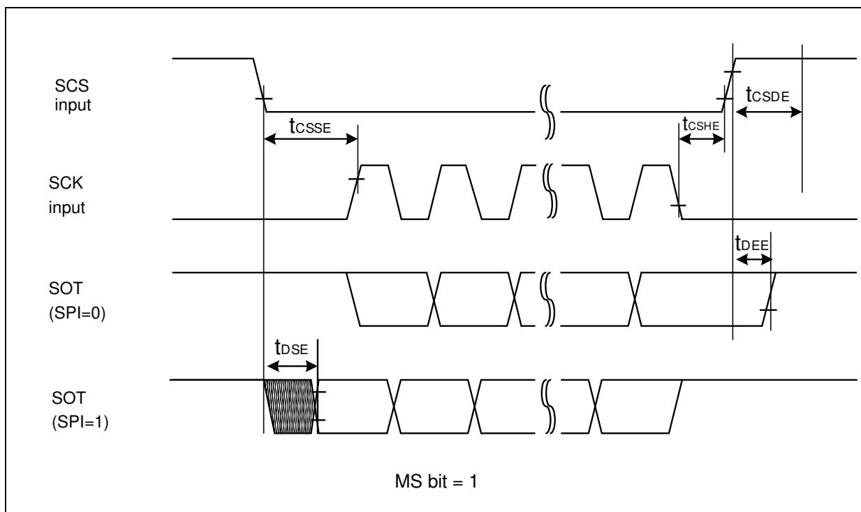
**When Using Synchronous Serial Chip Select (SCINV = 0, CSLVL=0)**
