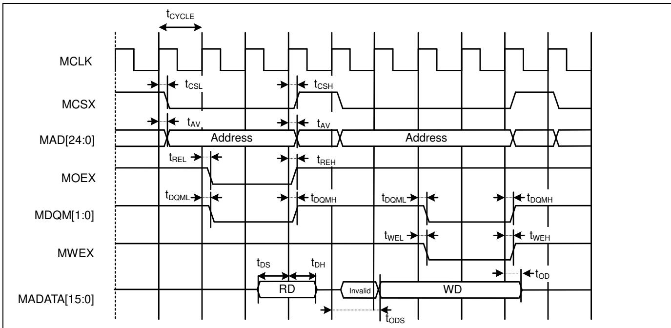
**Multiplexed Bus Access Asynchronous SRAM Mode**
