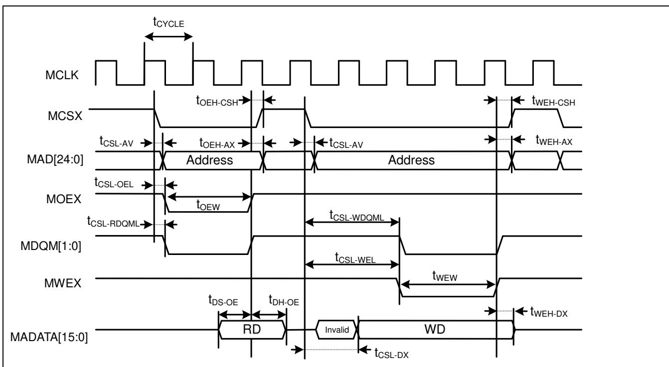
**Separate Bus Access Synchronous SRAM Mode**
