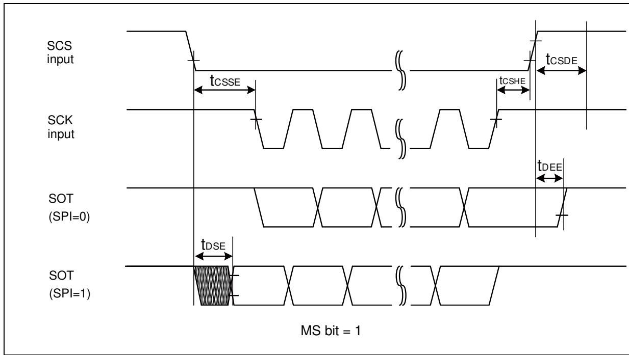
**When Using Synchronous Serial Chip Select (SCINV = 1, CSLVL=1)**
