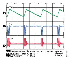
Figure 36. Typical Waveforms, V<sub>OUT1</sub> = 1.8 V, I<sub>OUT1</sub> = 30 mA, Auto Mode
