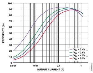
Figure 22. Buck Efficiency vs. Load Current, Across Input Voltage,  $V_{OUTI} = 1.8 V$ , PWM Mode
