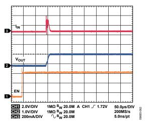
Figure 62. LDO1, LDO2 Startup, Vout = 1.2 V, Iout = 5 mA
