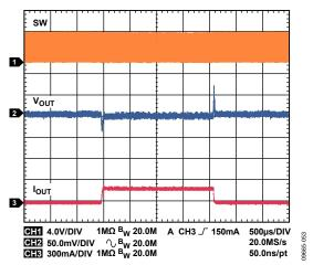
Figure 53. Buck Response to Load Transient,  $I_{OUT1} = 20$  mA to 200 mA,  $V_{OUT1} = 3.3$  V, PWM Mode
