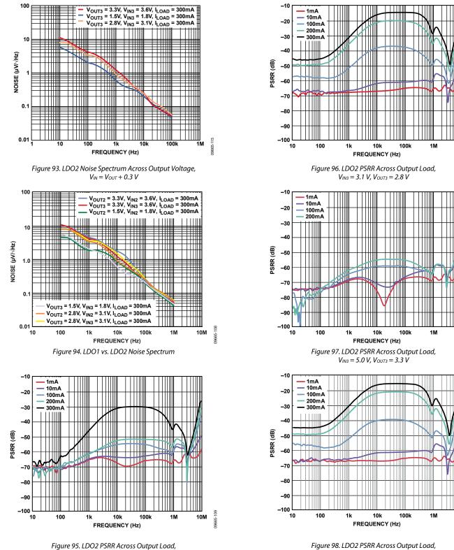
5. LDO2 PSRR Across Output Load,  $V_{IN3} = 3.3 V, V_{OUT3} = 2.8 V$  Figure 98. LDO2 PSRR Across Output Load,  $V_{IN3} = 3.6 V$ ,  $V_{OUT3} = 3.3 V$
