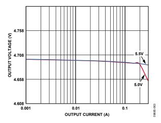
Figure 63. LDO1, LDO2 Load Regulation Across Input Voltage, VOUT = 4.7 V
