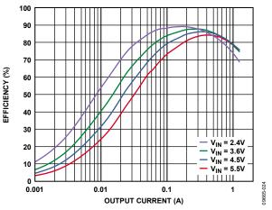
Figure 24. Buck Efficiency vs. Load Current, Across Input Voltage, V<sub>OUT1</sub> = 1.2 V, PWM Mode
