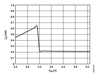
Figure 5. System Quiescent Current (Sum of All the Input Currents) vs. Input Voltage, V<sub>OUT1</sub> = 1.8 V, V<sub>OUT2</sub> = V<sub>OUT3</sub> = 3.3 V (UVLO = 3.3 V)
