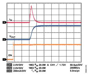
Figure 59. LDO1, LDO2 Startup, Vout = 4.7 V, Iout = 5 mA
