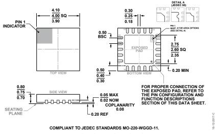
Figure 110. 20-Lead Lead Frame Chip Scale Package [LFCSP] 4 mm × 4 mm Body and 0.75 mm Package Height (CP-20-8) Dimensions shown in millimeters
