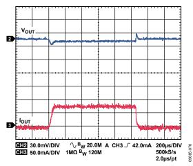
Figure 78. LDO1, LDO2 Response to Load Transient,  $I_{\text{OUT}}$  from 1 mA to 80 mA,  $V_{\text{OUT}}$  = 3.3 V
