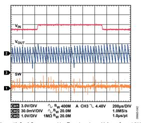
Figure 42. Buck Response to Line Transient, Input Voltage from 4.5 V to 5.0 V, V<sub>0UT1</sub> = 1.8 V, I<sub>0UT1</sub> = 5 mA, Auto Mode
