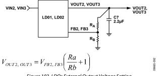
Figure 103. LDOs External Output Voltage Setting
