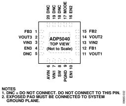
Figure 2. Pin Configuration—View from Top of the Die
