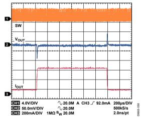
Figure 58. Buck Response to Load Transient,  $I_{OUT1} = 50$  mA to 500 mA,  $V_{OUT1} = 1.2$  V, PWM Mode
