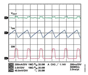
Figure 40. Typical Waveforms, V<sub>OUT1</sub> = 1.2 V, I<sub>OUT1</sub> = 30 mA, PWM Mode
