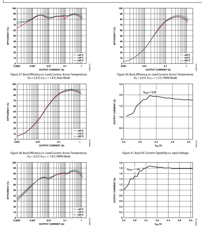
Figure 32. Buck DC Current Capability vs. Input Voltage
