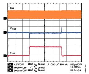
Figure 56. Buck Response to Load Transient,  $I_{OUT1} = 50$  mA to 500 mA,  $V_{OUT1} = 1.8$  V, PWM Mode
