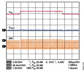
Figure 46. Buck Response to Line Transient, Input Voltage from 4.5 V to 5.0 V,  $V_{OUTI} = 1.2$  V, PWM Mode
