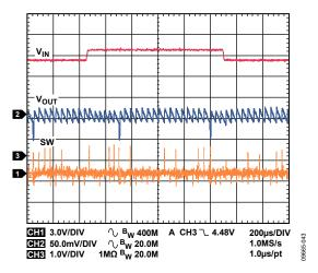
Figure 43. Buck Response to Line Transient, Input Voltage from 4.5 V to 5.0 V, V<sub>0UT1</sub> = 1.2 V, I<sub>0UT1</sub> = 5 mA, Auto Mode
