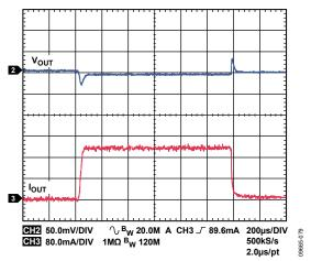
Figure 79. LDO1, LDO2 Response to Load Transient,  $I_{\rm OUT}$  from 10 mA to 200 mA,  $V_{\rm OUT}$  = 3.3 V
