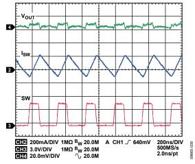
Figure 39. Typical Waveforms, V<sub>OUT1</sub> = 1.8 V, I<sub>OUT1</sub> = 30 mA, PWM Mode
