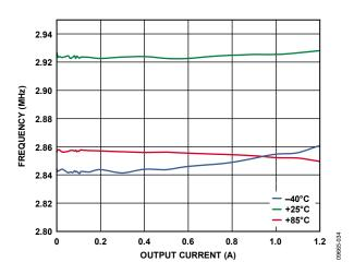
Figure 34. Buck Switching Frequency vs. Output Current, Across Temperature,  $V_{OUT1} = 1.8$  V, PWM Mode
