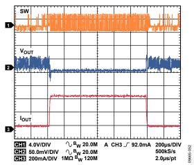
Figure 52. Buck Response to Load Transient,  $I_{OUT1} = 50$  mA to 500 mA,  $V_{OUT1} = 1.2$  V, Auto Mode
