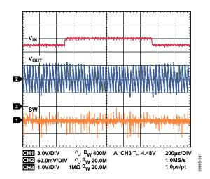
Figure 41. Buck Response to Line Transient, Input Voltage from 4.5 V to 5.0 V, V<sub>0UT1</sub> = 3.3 V, I<sub>0UT1</sub> = 5 mA, Auto Mode
