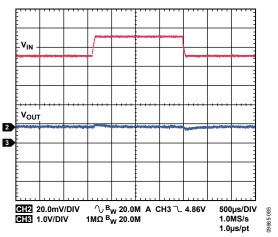
Figure 85. LDO1, LDO2 Response to Line Transient, Input Voltage from 4.5 V to 5.5 V,  $V_{OUT}$  = 1.8 V
