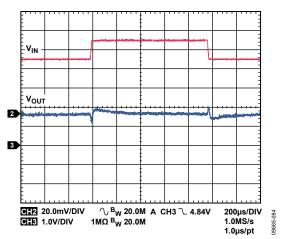
Figure 84. LDO1, LDO2 Response to Line Transient, Input Voltage from 4.5 V to 5.5 V,  $V_{OUT} = 3.3$  V
