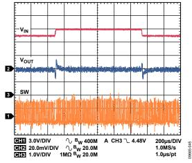
Figure 45. Buck Response to Line Transient, Input Voltage from 4.5 V to 5.0 V, Vouti = 1.8 V, PWM Mode
