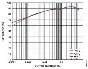
Figure 25. Buck Efficiency vs. Load Current, Across Temperature,  $V_{IN} = 5.0 V$ ,  $V_{OUTI} = 3.3 V$ , Auto Mode
