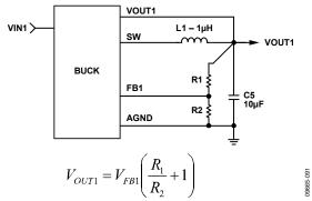
Figure 102. Buck External Output Voltage Setting
