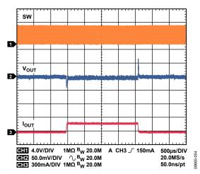
Figure 54. Buck Response to Load Transient,  $I_{OUT1} = 50$  mA to 500 mA,  $V_{OUT1} = 3.3$  V, PWM Mode
