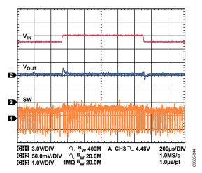
Figure 44. Buck Response to Line Transient, Input Voltage from 4.5 V to 5.0 V,  $V_{OUTI} = 3.3$  V, PWM Mode
