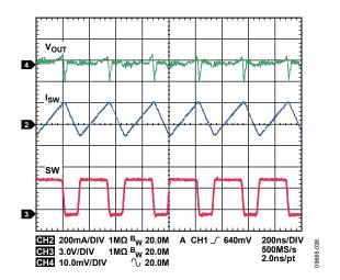
Figure 38. Typical Waveforms, Vouti = 3.3 V, Iouti = 30 mA, PWM Mode
