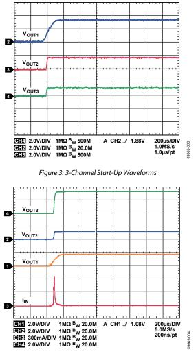
Figure 4. Total Inrush Current, All Channels Started Simultaneously
