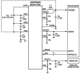
Figure 106. Processor System Power Management with PSM/PWM Control
