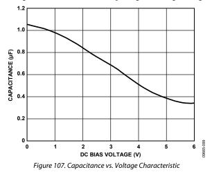
Use the following equation to determine the worst-case capacitance accounting for capacitor variation over temperature, component tolerance, and voltage.
