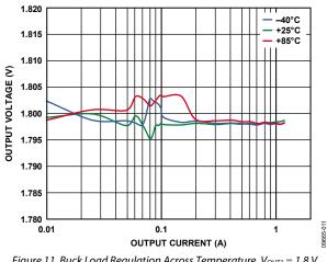
Figure 11. Buck Load Regulation Across Temperature,  $V_{OUT1} = 1.8 V$ , Auto Mode
