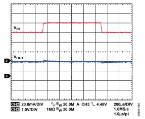
Figure 86. LDO1, LDO2 Response to Line Transient, Input Voltage from 4.5 V to 5.5 V, V<sub>OUT</sub> = 1.2 V
