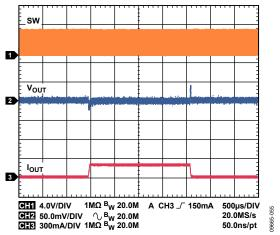
Figure 55. Buck Response to Load Transient,  $I_{OUT1} = 20$  mA to 200 mA,  $V_{OUT1} = 1.8$  V, PWM Mode
