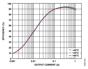
Figure 26. Buck Efficiency vs. Load Current, Across Temperature,  $V_{IN} = 5.0 V$ ,  $V_{OUT1} = 3.3 V$ , PWM Mode
