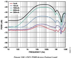
Figure 100. LDO1 PSRR Across Output Load,  $V_{IN2} = 1.8 V$ ,  $V_{OUT2} = 1.5 V$
