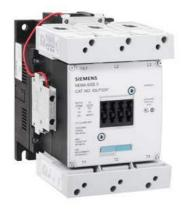
Vacuum NEMA contactor, Size 5, Three phase full voltage, Contactor amp rating 270A, 3 wire (NO aux included), 200-220V 50-60Hz/DC coil, Non-combination type, Enclosure NEMA type (open), No enclosure
