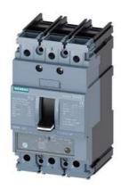
circuit breaker 3VA5 UL frame 125 breaking capacity class S 25kA @ 480 V 3-pole, line protection TM240, ATAM, In=30A overload protection Ir=24A ...30A short-circuit protection li=5...10 x In cable connection on both sides
