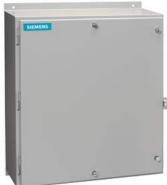
Non-reversing motor starter, Size 3, Three phase full voltage, Solid-state overload relay, OLRelay amp range 25-100A, 208VAC 60HZ coil, Non-combination type, Enclosure type 12, Dust/drip proof for indoors, Extra-wide enclosure
