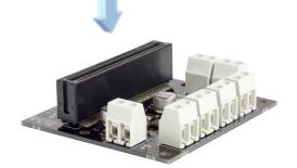
Inserting a BBC micro:bit: To use the motor driver board the BBC micro:bit should be inserted firmly into the connector as shown left.
