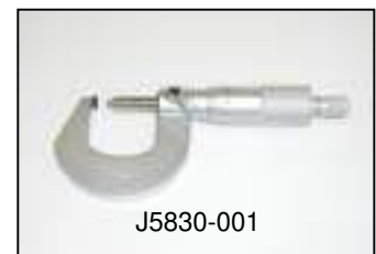
Measurement of crimp height of conductor wire
