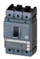
circuit breaker 3VA5 UL frame 250 breaking capacity class H 65kA @ 480 V 3-pole, line protection TM210, FTFM, In=70A overload protection Ir=70A fixed short-circuit protection li=10 x In nut keeper kit on both sides
