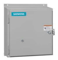
Non-reversing NEMA contactor, Size 1, Three phase full voltage, Contactor amp rating 27A, 3 wire (NO aux included), 190-220/220-240V 50/60Hz coil, Noncombination type, Encl. NEMA type 4X fiberglass, Water/dust tight noncorrosive, Standard width enclosure
