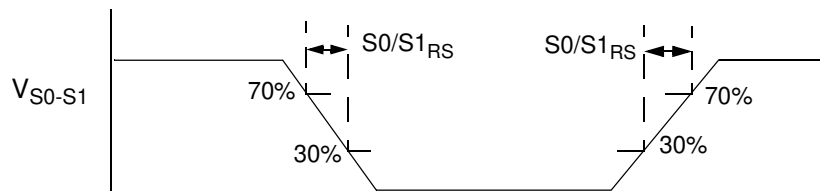
Figure 6. Slew Time Measurement
