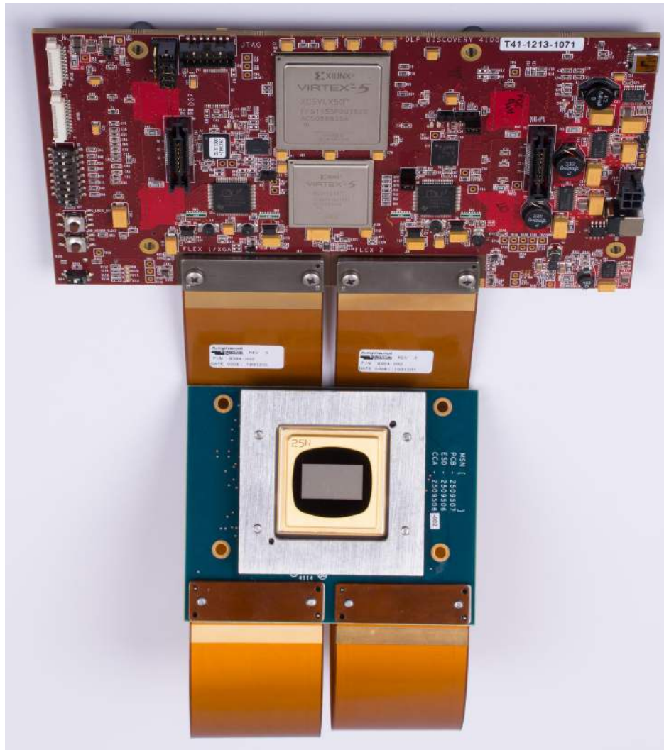
Figure 2-2. DLPLCRC410EVM connected to DLPLCR95EVM
