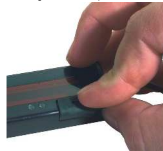
Figure 7. Cover Replacement – Pressing Cover
