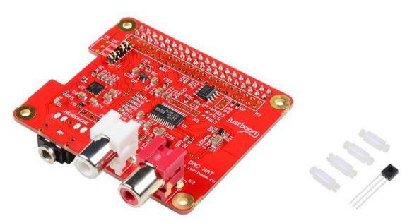
The JustBoom DAC HAT is a plug-and-play, high-resolution, digital-to-analog converter for the Raspberry Pi. Simply stack the plug-and-play add-on board (HAT) onto your Raspberry Pi A+, B+, 2B or the new 3B, and it will be ready to use immediately.
