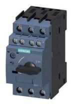
Circuit breaker size S00 for motor protection, CLASS 10 A-release 7...10 A N release 130 A screw terminal Standard switching capacity with transverse auxiliary switches 1 NO+1 NC
