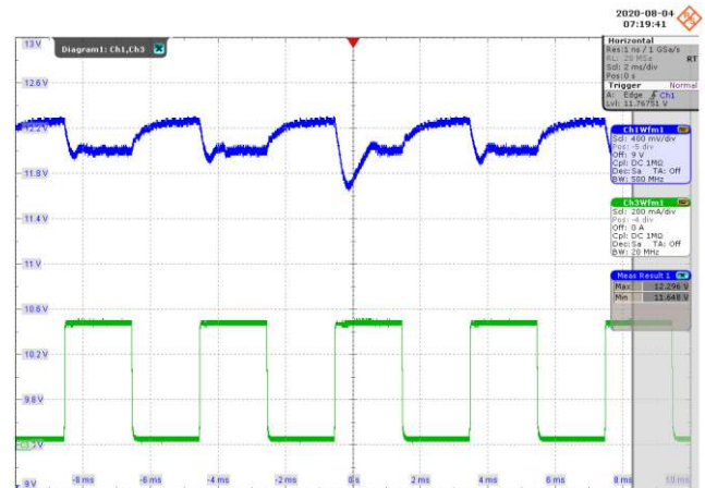
Figure 90 – Transient Output Waveforms. 115 VAC. Upper: V_{OUT} , 400 mV / div., 2 ms / div. Lower: I_{OUT} 200 mA / div. Load Transient: 5 % - 100%. Duty Cycle, Slew Rate: 50%, 0.8 A / \mu s. Frequency: 250 Hz. V_{MAX} : 12.30 V, V_{MIN} : 11.65 V.
