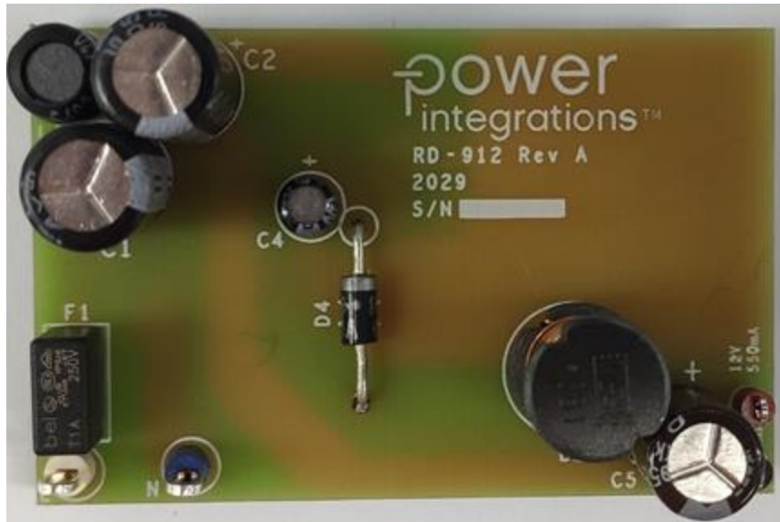
Figure 1– Populated Circuit Board Photograph, Top.
