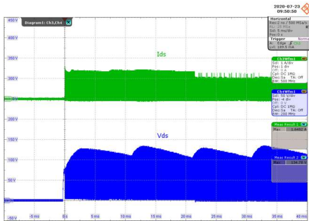
Figure 26 – Drain Voltage and Current Waveforms. 85 VAC, 550 mA Output. Upper: I_{DS} , 1 A / div. Lower: V_{DS} , 50 V / div., 5 ms / div. I_{DS(MAX)} = 1.65 A, V_{DS(MAX)} = 134.8 V.
