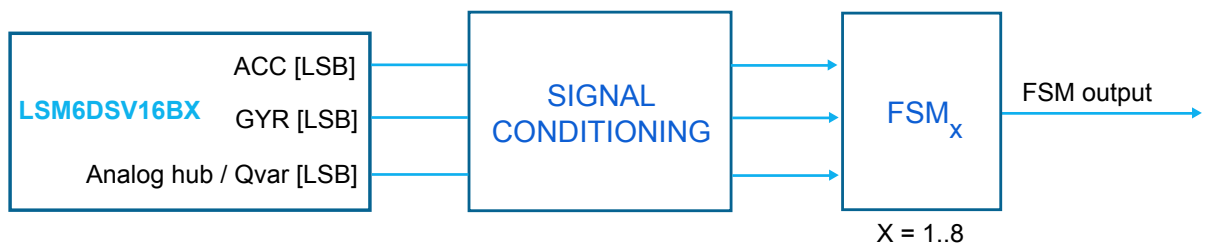
Figure 3. State machine in the LSM6DSV16BX
