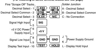
**Pins A, 1 and 3 - Decimal Select:** Decimal points may be blanked as required by carefully scraping off the fine tracks linking these pins to Decimal Select Common using a pair of pliers or a small screwdriver blade. Re-connect either by linking the appropriate pins on the connector or by solder-bridging the junctions located on the PC board edge fingers.
