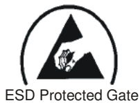
ESD Protected Gate
