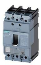
circuit breaker 3VA5 UL frame 125 3-pole, starter protection TM120M, AM, In=40A without overload protection short-circuit protection Ii=3...7 x In cable connection on both sides
