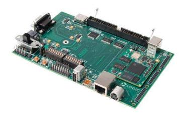
Congratulations on your purchase of the Zoom AM3517 eXperimenter Kit. This Zoom Development Kit provides a product-ready hardware and software platform for evaluating the functionality of the Texas Instruments (TI) AM3517 processor and the Logic PD System on Module (SOM).
