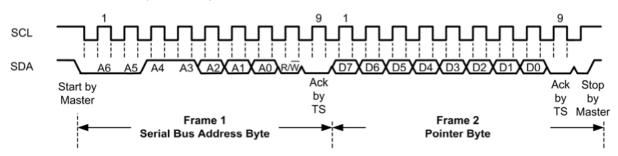
SMBus/I<sup>2</sup>C write to the pointer register followed by a write data word
