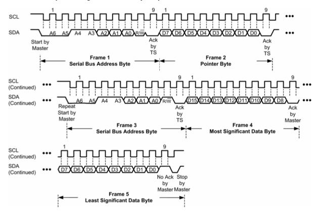
SMBus/I<sup>2</sup>C write to pointer register followed by a repeat start and an immediate data word read
