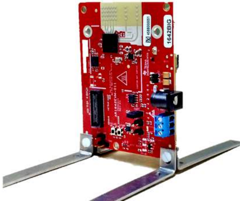
Figure 22. Vertical Assembly of EVM
