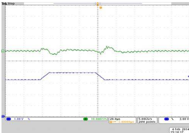
Figure 14. Line Transient, 5 mA Load, 10 µs Step
