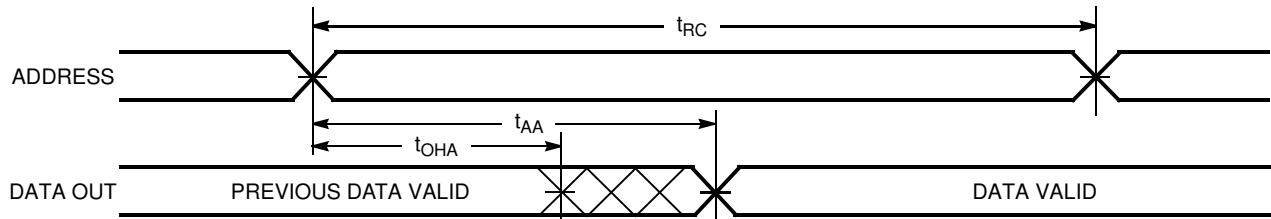
Read Cycle No. 2 ( $\overline{OE}$  Controlled)<sup>[16, 17]</sup>
