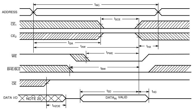
Write Cycle No. 3 ( $\overline{\text{WE}}$  Controlled,  $\overline{\text{OE}}$  LOW)<sup>[19]</sup>
