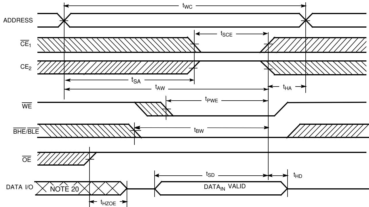
Write Cycle No. 3 ( $\overline{WE}$  Controlled,  $\overline{OE}$  LOW)<sup>[19]</sup>
