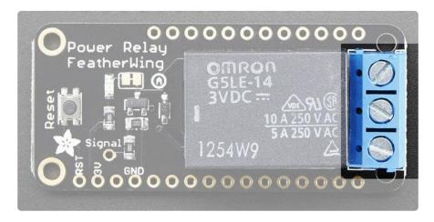
The Wing has the power control output on the end, a 3-pin 5.08 mm terminal block. The COM pin is what you should connect the signal you're planning to switch.
