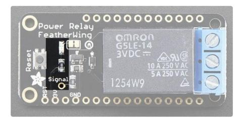
Controlling the relay is really simple. The relay uses a single pin for control. When floating or pulled low, the relay is 'open' or unset. When the pin is pulled high, the relay switches closed/set. A red LED next to the pin will let you know that the signal is high. You will need to solder closed a jumper on the bottom to match the pin you want to use for control.
