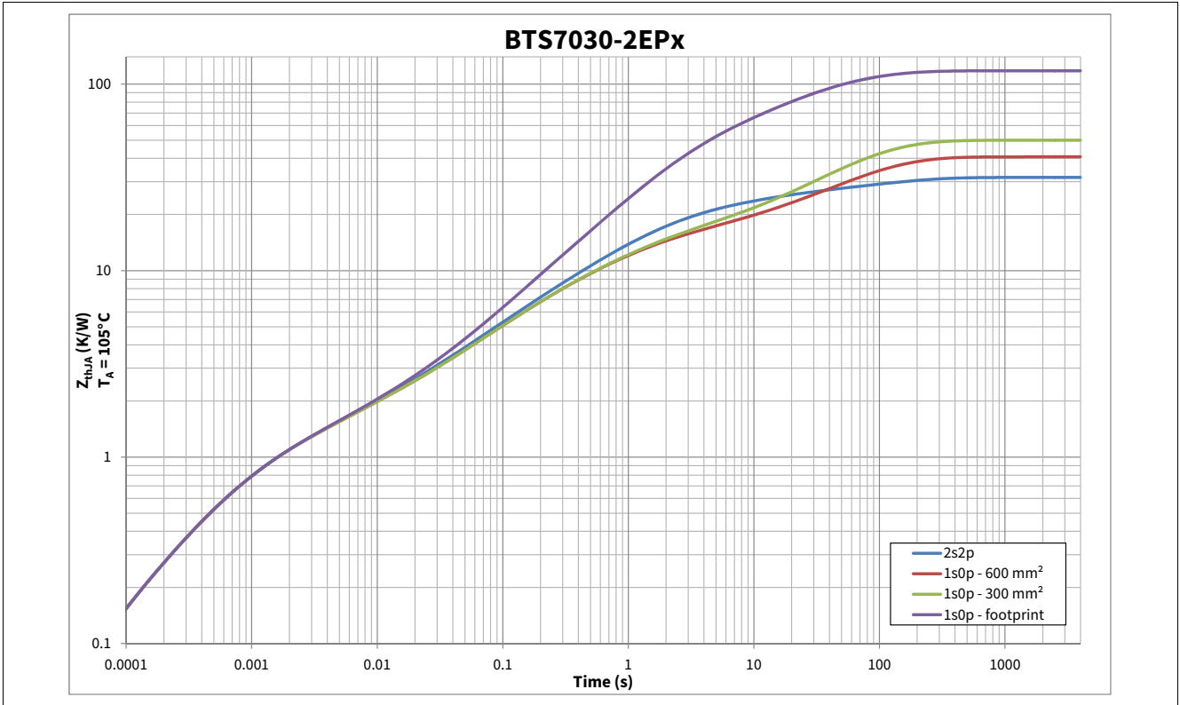
Figure 9 Typical Thermal Impedance. PCB setup according Chapter 4.4.1
