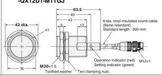
\*1. The E2EF-QX\(\subseteq\)D type Clamping nut (optional accessory) is grooved to identify the material (SUS303, with fluororesin coating).
