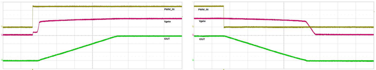
Figure 16: Rise Time and Fall Time During PWM Dimming. I OUT (Total LED Current) (200 mA/div), PWM_IN and V GATE (2 V/div), Time (20 μs/div)
