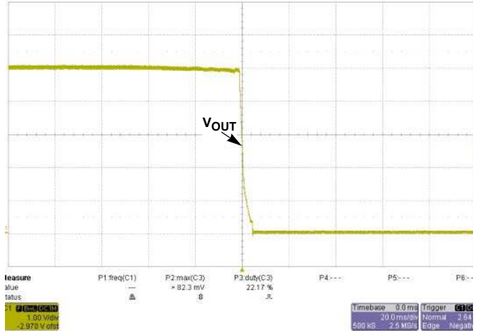
FIGURE 18. SHUT-DOWN AT V_{IN} = 75V @ I_O = 40A
