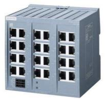
$\label{eq:scalarse} \begin{array}{l} \text{SCALANCE XB124 unmanaged IE switch, 24x 10/100 Mbit/s RJ45 ports;} \\ \text{for setting up small star and line topologies; LED diagnostics, IP20,} \\ \text{Redundant power supply, 24 V AC/DC Manual available as a download} . \end{array}$
