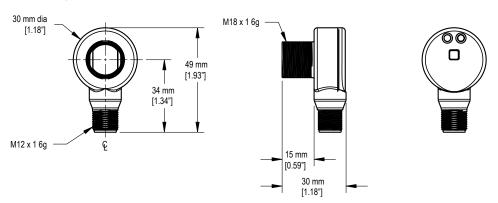
Maximum Torque specification: 5.6 nm or 50 in-lbs. Lockwasher and M18 nut included.
