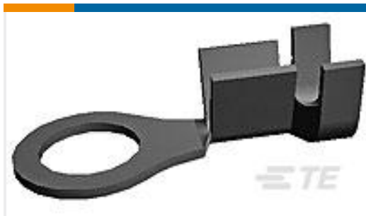
TE Part #40955 RING 20-16 AWG .0295 X .390 TPBR
