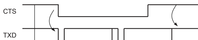
Figure 38-28: Transmitter Behavior when Operating with Hardware Handshaking
