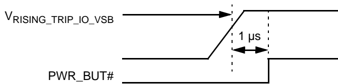
Figure 7-12. Skip Electrical Parameters
