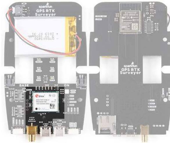
Two internal slide switches control the flow of NMEA and RTCM traffic between the external connectors and the internal BT UART used on the ESP32. Ostensibly the *Bluetooth Broadcast* switch can be set to pipe RTCM data to the ESP32's UART (instead of NMEA) so that correction data can be transmitted over Bluetooth. Point to point Bluetooth radio support is not supported because the useful range of Bluetooth is too short for most RTK applications but may be helpful in some advanced applications.
