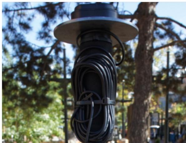
*u-blox L1/L2 antenna with ground plate*
