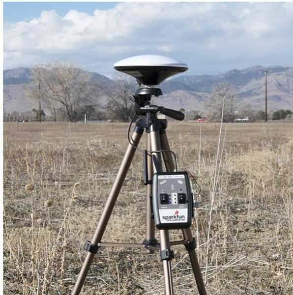
*Temporary RTK Surveyor Base setup*
