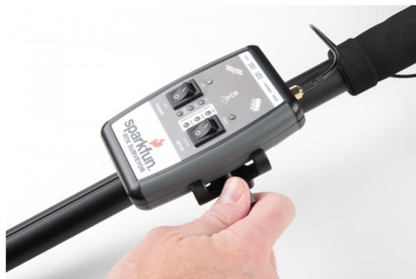
If you are receiving RTCM correction data over a radio link it's recommended that you attach a radio to the back of the RTK Surveyor.
