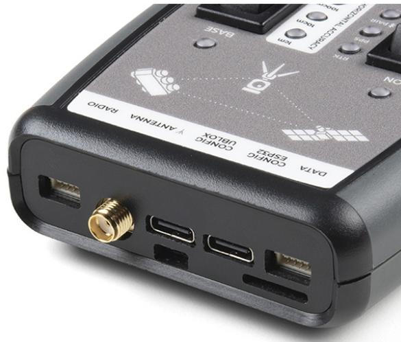
*The SparkFun RTK Surveyor has a variety of connectors*
