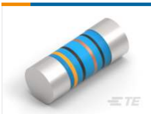
TE Part #1-2176315-3 MELF SMA_A 1K0 0.1% 15PPM 0204 0.4W
