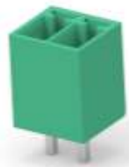
TE Part #2351886-2 2POS TB HDR 180 DEG, PITCH 3.5, TL 3.4mm
