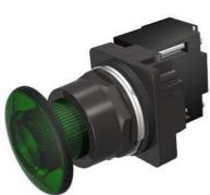
30mm BlackMax, Epoxy Coated Corrosion Resistant Complete Metal Unit Illuminated Push-Pull Operator Transformer type, 240V AC Incandescent Lamp Mushroom Head Cap Small 1 3/4" (44.5 mm) Plastic, Green 3 Position Pull-Momentary/Push-Maintained UL Listed, CSA Certified NEMA 1,3,3R,4,4X,12,13 & Automotive Standards
