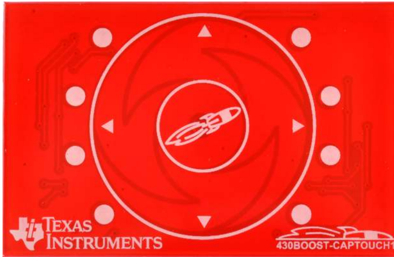
Figure 6. Capacitive Touch BoosterPack Hardware
