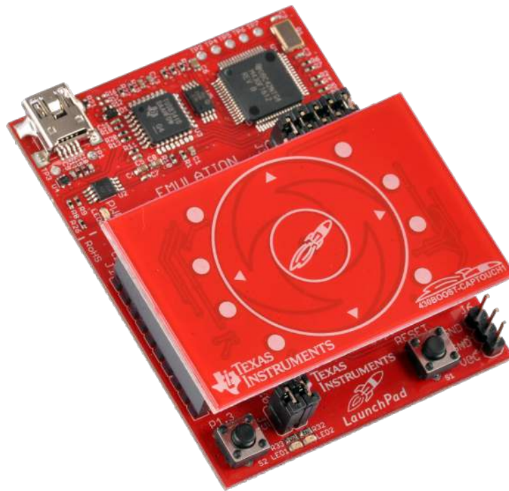
Figure 1. Capacitive Touch BoosterPack With LaunchPad
