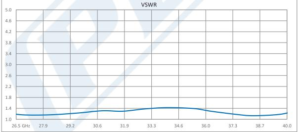
Click the following link (or enter part number in "SEARCH" on website) to obtain additional part information including price, inventory and certifications: Isolator with 12 dB Isolation from 26.5 GHz to 40 GHz, 10 Watts and 2.92mm Female PE83IR1036
