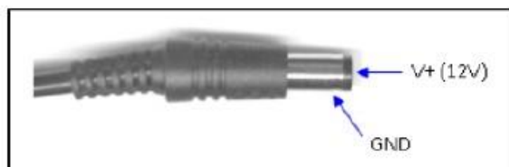
Figure 3: 2.1 mm Power Connector
