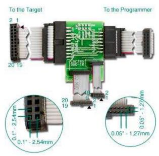
ChipProg-ISP BH14/BH20 and BH10 specialized adapter for in system programming of ARM microcontrollers .
