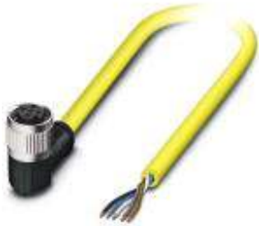
Sensor/Actuator cable, 5-position, TPE, yellow RAL 1021, free cable end, on Socket angled M12 SPEEDCON, A-coded, Cable length: 2 m
