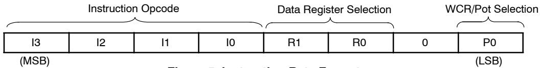
Figure 5. Instruction Byte Format
