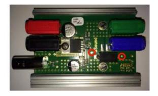
The voltage drop over the resistance (R1) can be measured between the test points TP1 and TP5 (marked in red) or directly at the resistance. The current through the load can then be calculated with the following formula:
