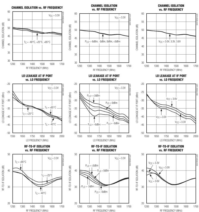
**high-side injected** for a 350MHz IF,  $P_{RF} = -5dBm$ ,  $P_{LO} = 0dBm$ ,  $T_C = +25^{\circ}C$ , unless otherwise noted.)
