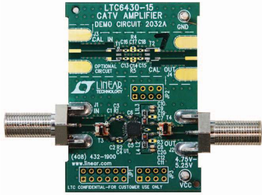
Figure 17. LTC6430-15 CATV Evaluation Board
