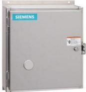
Non-reversing NEMA contactor, Size 2, Three phase full voltage, Contactor amp rating 45A, 3 wire (NO aux included), 380-440/440-480V 50/60Hz coil, Noncombination type, Encl NEMA type 4X 304 S-Steel, Water/dust tight noncorrosive, Extra-wide enclosure
