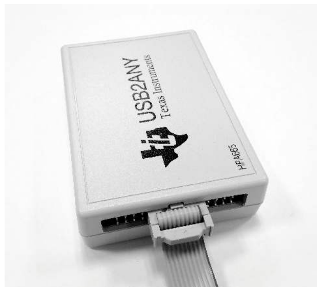
Figure 6. Ribbon Cable Connected to the Ten Middle Pins of the USB2ANY Interface Adapter
